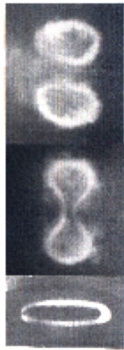
AR=4, laboratory jet flow visualization Hussain & Husain, JFM (1989).
