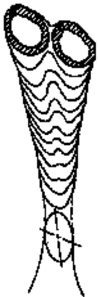
AR=4, laboratory jet flow visualization Hussain & Husain, JFM (1989).
